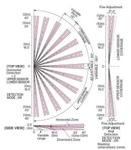
Detection distance is set by adjusting the angle of downward zone. Adjustable range 6.6' (2m) to 40' (12m). [10 ranges]
