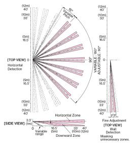
Detection distance is set by adjusting the angle of downward zone. Adjustable range 6.6' (2m) to 40' (12m). [10 ranges]
