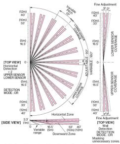
Detection distance is set by adjusting the angle of downward zone. Adjustable range 6.6' (2m) to 40' (12m), [10 ranges]
