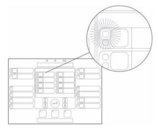
If Fire Alarm and Zone Alarm LEDs are flashing, the fire alarm has been activated by a detector. If they are steady, the fire alarm has been activated by a manual call point.
