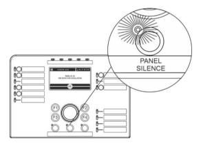
The Panel Silence LED turns on and the buzzer stops. New alarm or fault events will turn the buzzer back on.
