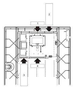
The inserts are numbered 1, 2, 3, and 4, and are inserted at the location indicated (with the printed area facing the front of the control panel).
