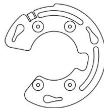
3. Place the metal PTZ adapter plate on the cup base. The arrow that states FRONT should be pointing away from the cup base. Using screw A, secure the adapter plate to the cup base. Tighten screw A fully, otherwise the dome will not slide properly into place over the three standoffs and the screw head will block the rotation.
