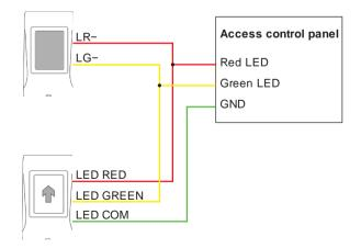
**Note:** The LED light can be controlled internally or externally (by LED wires). If switch 3 is OFF then the control of the light is left to the device itself. If switch 3 is ON, then the LED light is controlled by the device where the LED wires are connected.
