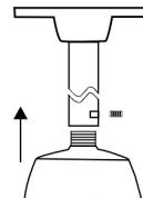
2. Remove the back box from the dome camera. It is not required when installing in a cup base.
