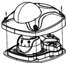
4. Install the mounting base to the surface using two of the M4 x 25 mm screws and anchors. If routing the cable harness through the ceiling, do so prior to mounting the camera.
