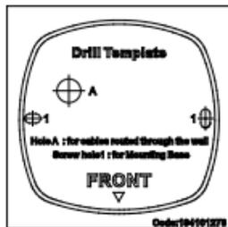
2. Follow all local safety regulations. Drill through the mounting surface. If you need to route the cables from the bottom of the camera, drill a larger hole in the mounting surface for the cable harness.
