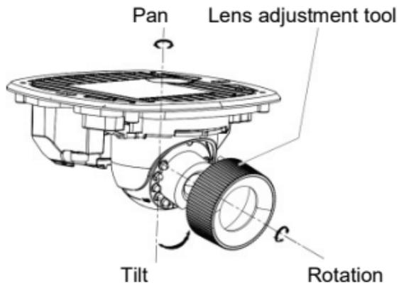
**Note:** Please do not remove the foam ring attached to the lens. This foam ring is required to reduce the glare of IR illuminators.
