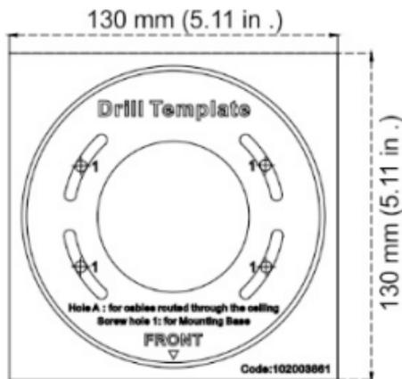
2. Follow all local safety regulations. Drill through the mounting surface. If you need to route the cables from the bottom of the camera, drill a larger hole for the cable harness.
