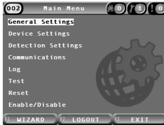
Figure 23: Access level 2 Main menu
