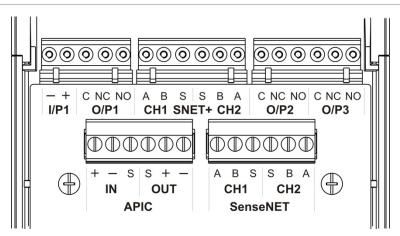
Figure 13: Backplane PCB connectors (bottom)
