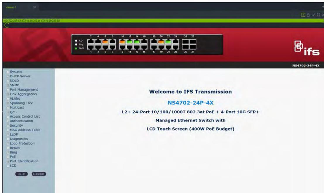
**Note:** If a switch is plugged into a switch via an RJ45 connector, it must be properly configured so that it appears in the Navigator panel. Go to **Port Identification > Configuration** in the switch's web UI and select **Switch** from the drop-down list next to the port number that the switch is connected to.
