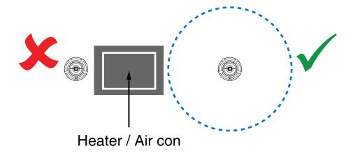
DO NOT install heat detectors directly above cookers, stoves, ovens, or in areas of high humidity such as bathrooms, shower rooms, or near dish washers and washing machines.
