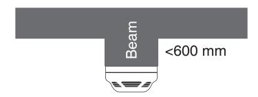
A detector should not be mounted within 500 mm of any obstruction or twice the depth of the beam, (whichever is less).
