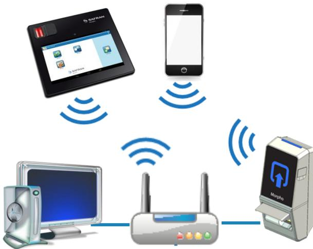
The connection to the embedded Webserver, through LAN or WLAN, requires terminals IP address and terminals password.
