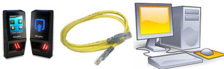
Figure 21: Direct Point to Point Ethernet Connection
