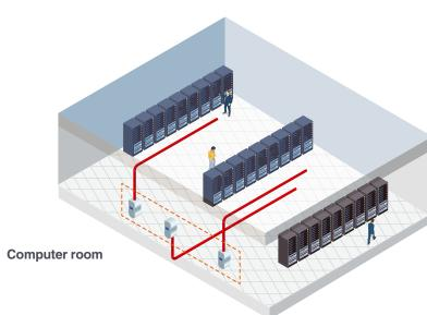
A VIP pass to any location. Equipment rooms housing high voltage machinery or sensitive computer equipment are generally secure areas with restricted access making servicing of smoke detection difficult. ModuLaser detector modules can be located outside of the risk area to overcome accessibility problems.
