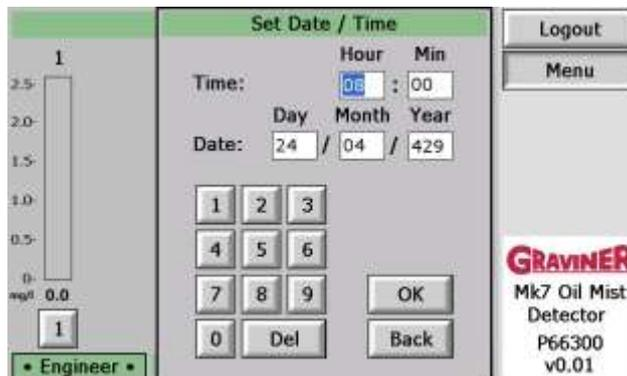
Figure 171 RTC Battery Failure
