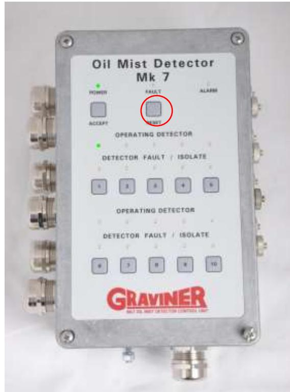
Press 'Reset' button for a minimum of 1sec
