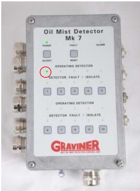
Current Modbus address flashing
