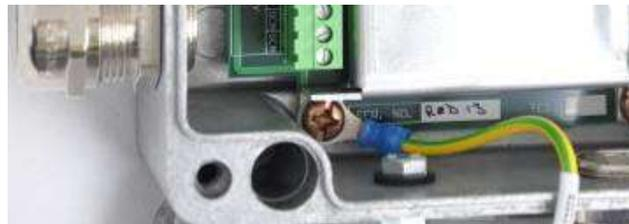
Figure 183 Control Unit Earth Wire
