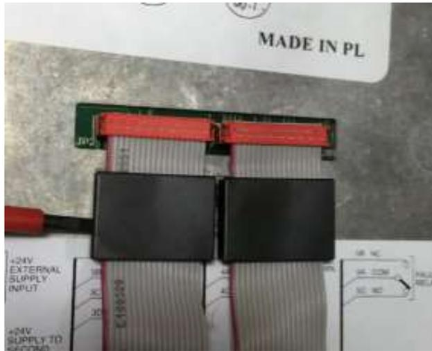
Figure 184 Ribbon Connector Ferrites
