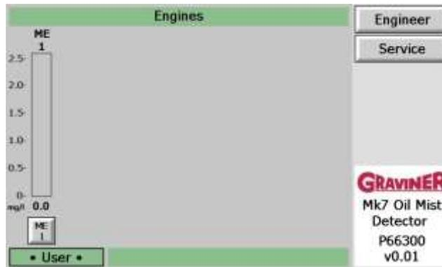
Figure 32 Engine Overview Screen – User Level
