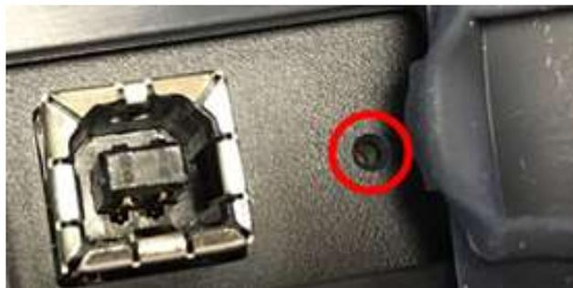
Figure 179 Remote Display Reset
