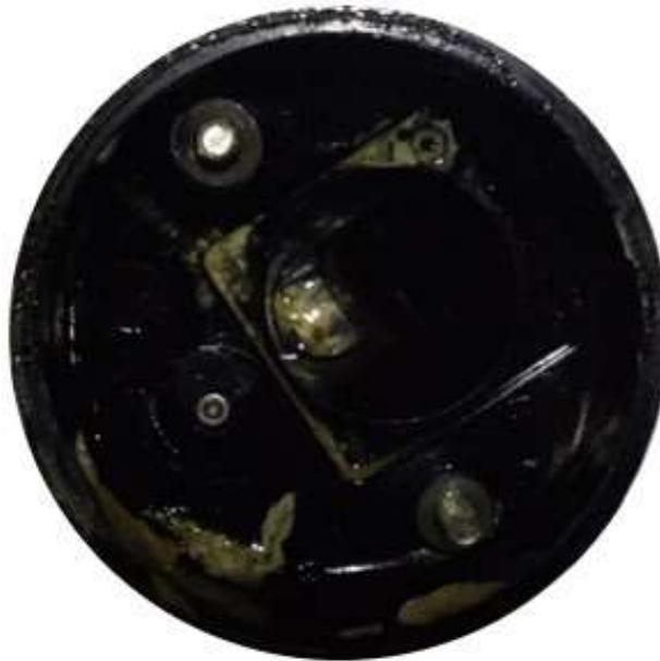
Figure 140 Emulsified oil in the detector base
