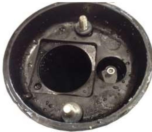
Figure 139 Water Droplets in the base.
