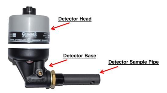
The oil mist detection chamber in each Detector Head must be inspected at regular intervals and cleaned to remove any buildup of oil splash or carbon deposits created by the operation of the engine.
