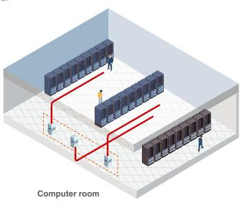
A VIP pass to any location. Equipment rooms housing high voltage machinery or sensitive computer equipment are generally secure areas with restricted access making servicing of smoke detection difficult. ModuLaser detector modules can be located outside of the risk area to overcome accessibility problems.
