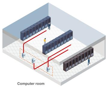
A VIP pass to any location. Equipment rooms housing high voltage machinery or sensitive computer equipment are generally secure areas with restricted access making servicing of smoke detection difficult. ModuLaser detector modules can be located outside of the risk area to overcome accessibility problems.
