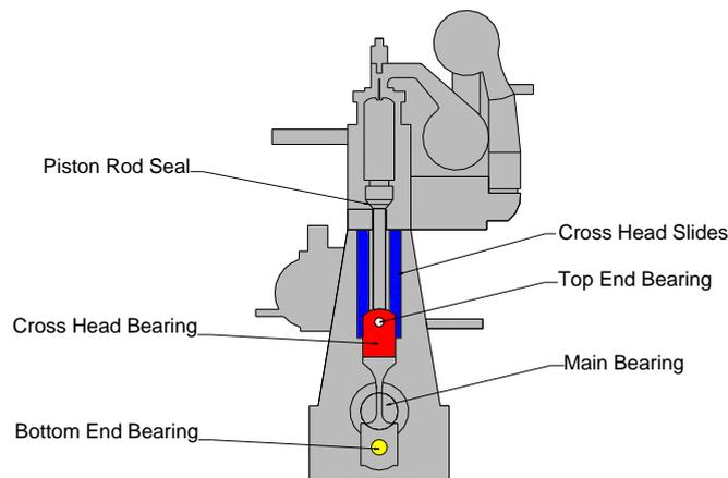
Figure 1 Areas of Failure – 2 Stroke Engine
