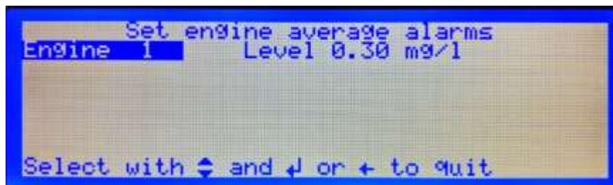
Figure 55 Set Engine Average Alarm
