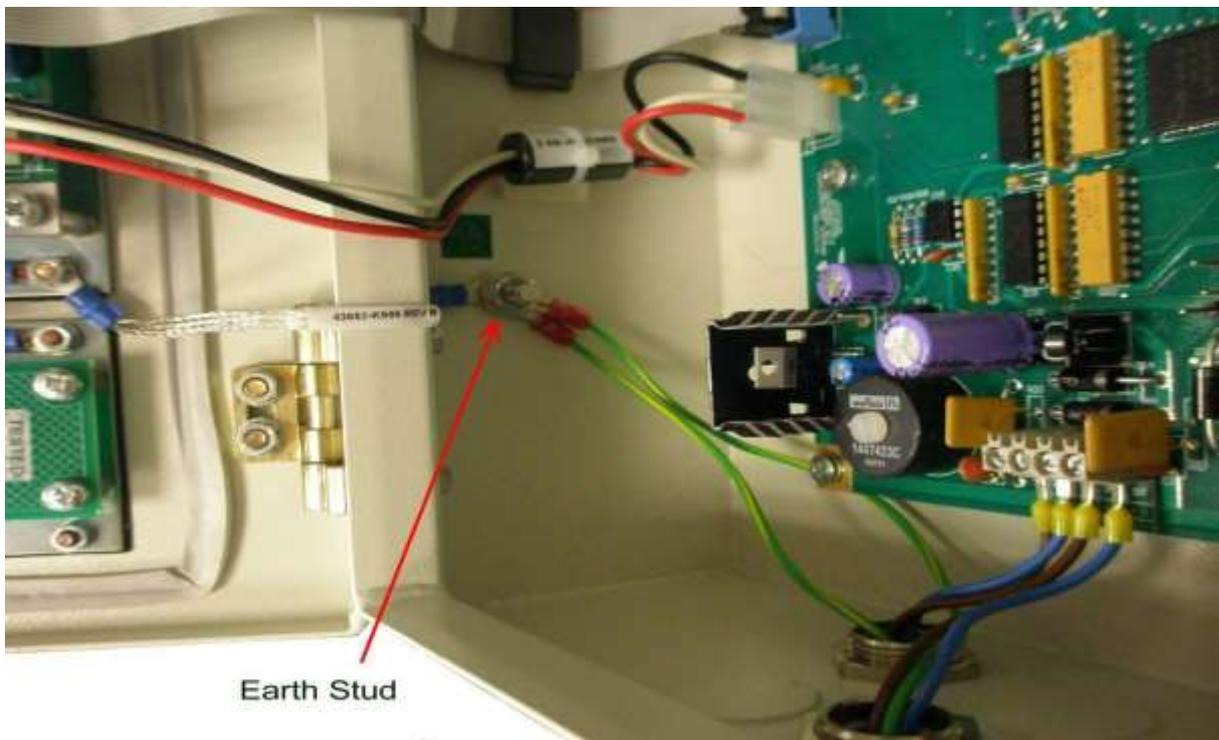
Figure 19 Power Input Cable Earth Stud
