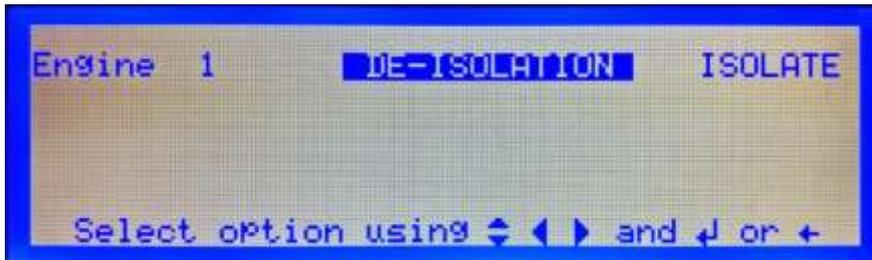
Figure 116 Isolate Engine
