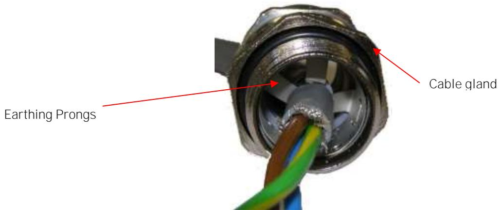
Figure 18 Power cable through EMC gland
