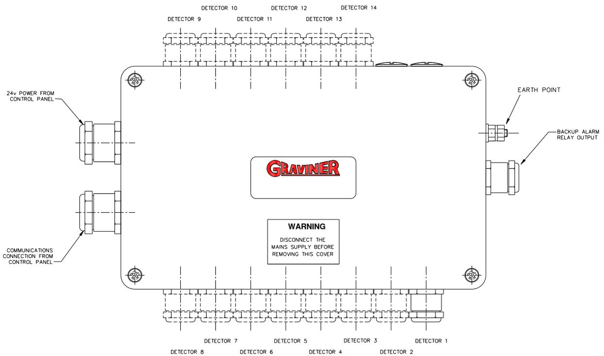
Figure 10 Junction Box External Connections
