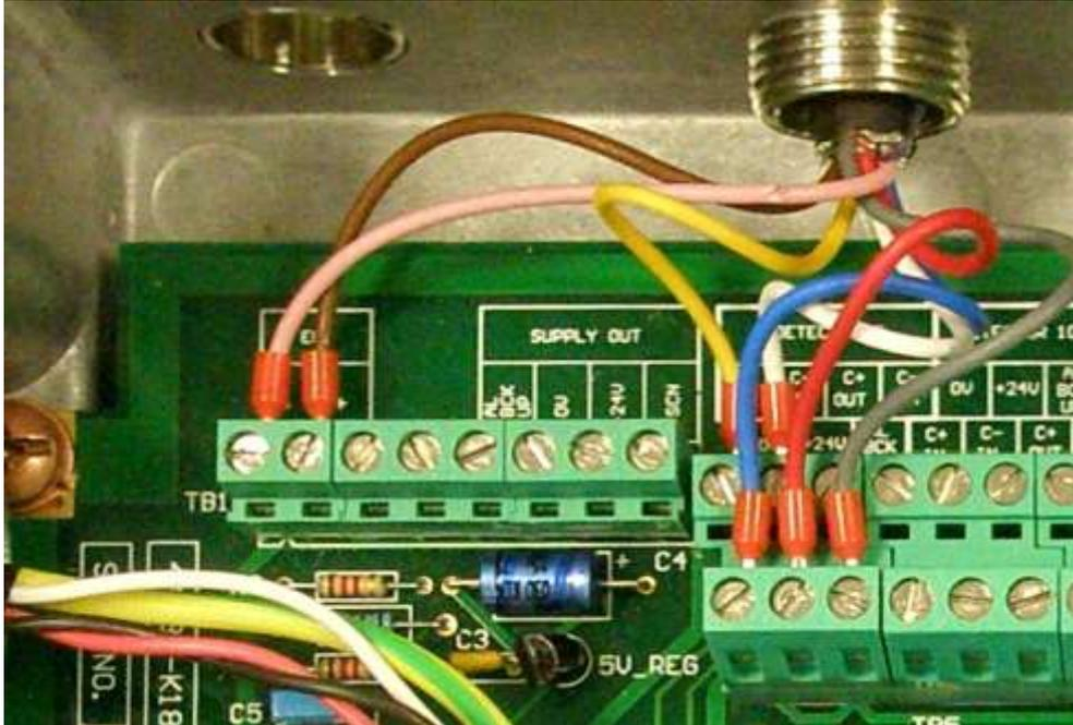
Figure 140 Communications End of Line Termination
