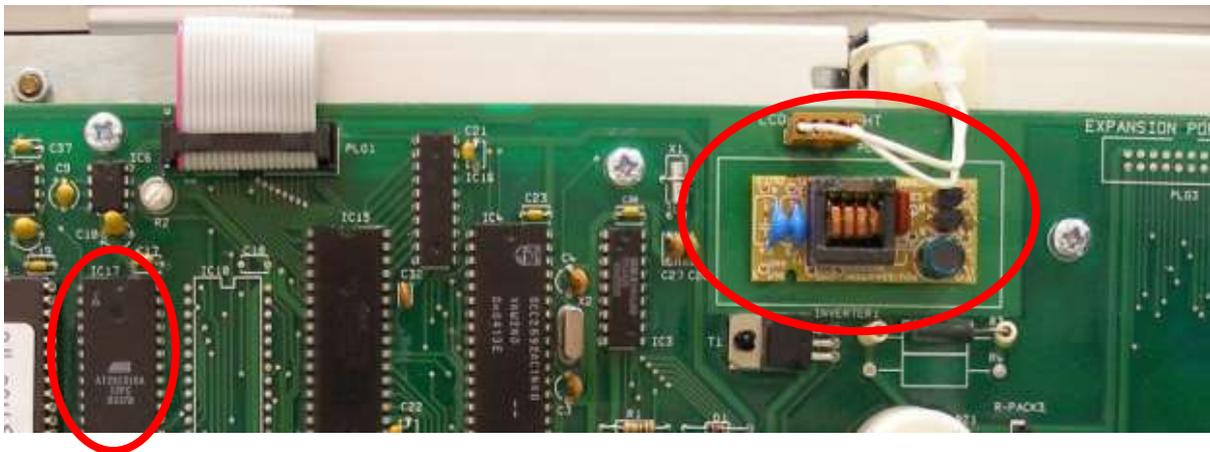
The original Control Panel display used a CCFL backlight that contained small amounts of mercury now prohibited by the RoHS directive.
