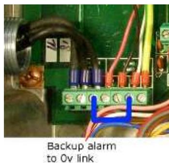
Figure 136 Link on Junction Box TB9
