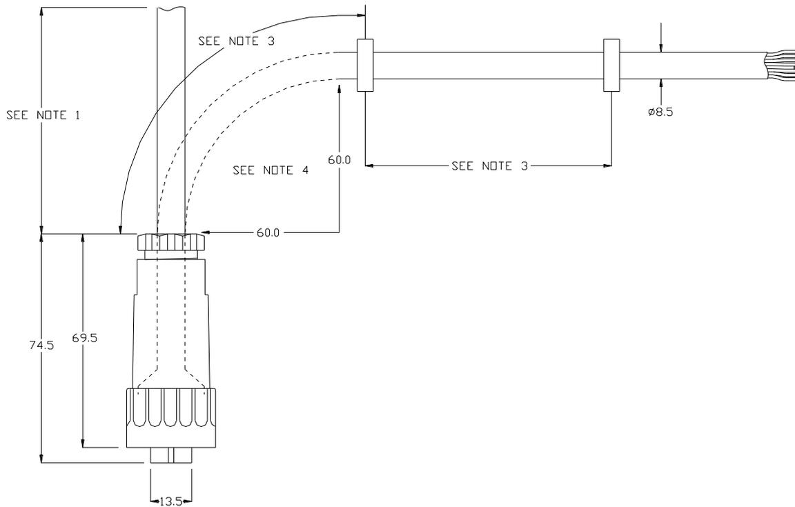
Figure 15 Detector Cable Assembly (Straight Connector)
