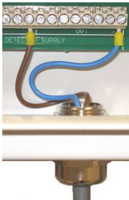
Figure 25 Power cable connections to I nterface Board.
