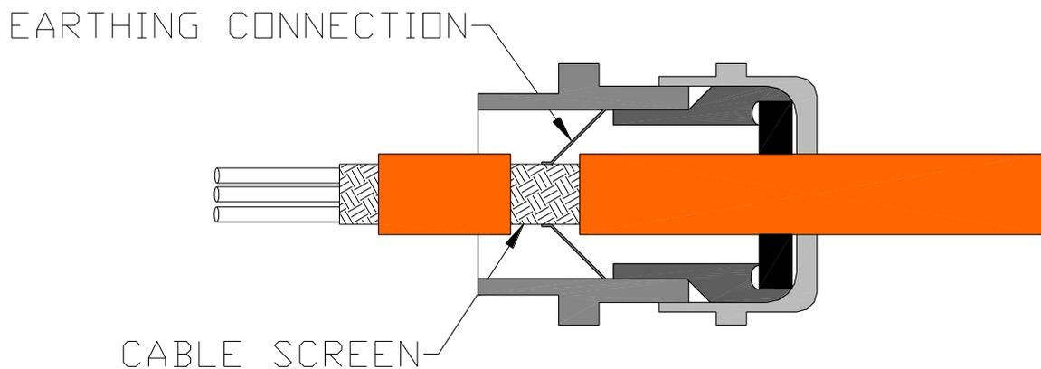
Figure 21 Control Panel relay cable assembly
