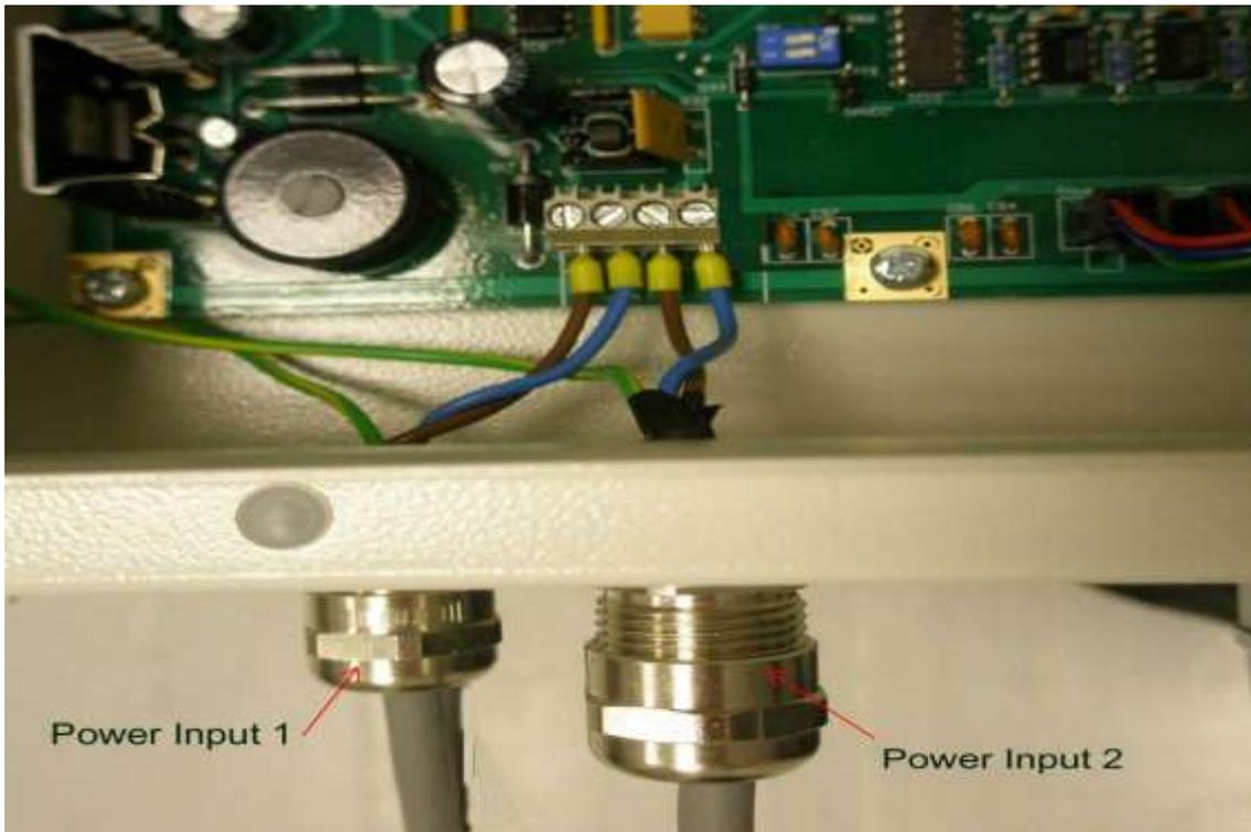
Figure 20 Power connections
