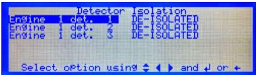
Figure 118 Detector Isolate – Detector Selection
