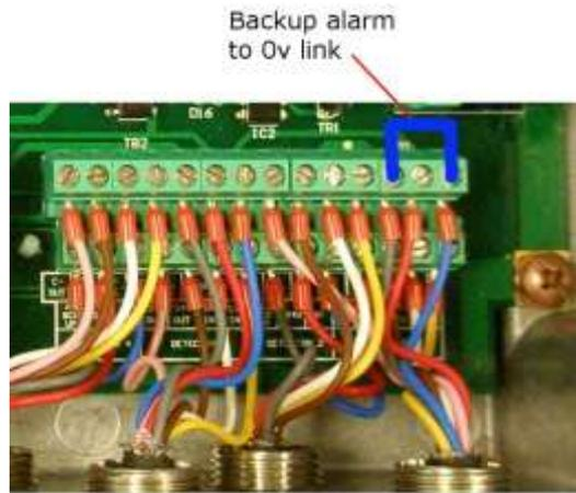
Figure 135 Link at Detector Connections
