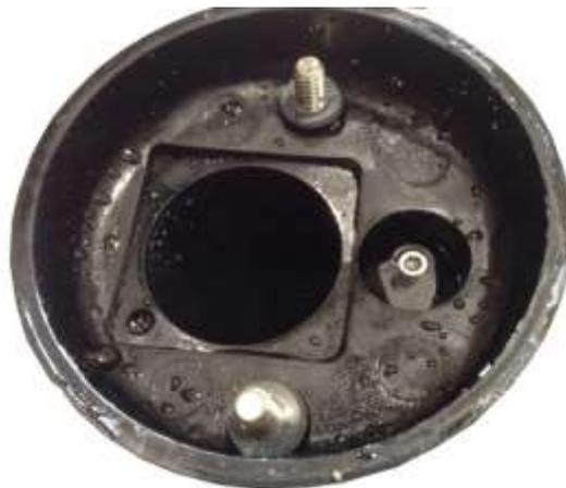
Figure 122 Water Droplets in the base.
