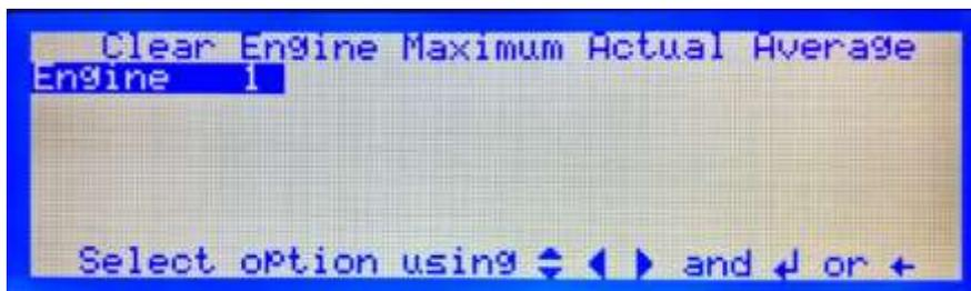
Figure 71 Clear Max Average Levels – Engine Selection
