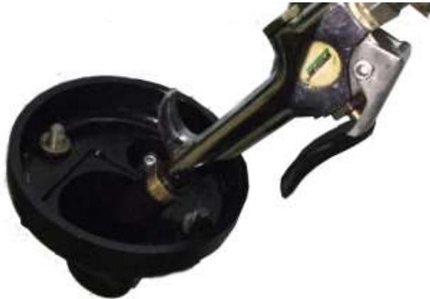
Figure 125 Detector Base Cleaning
