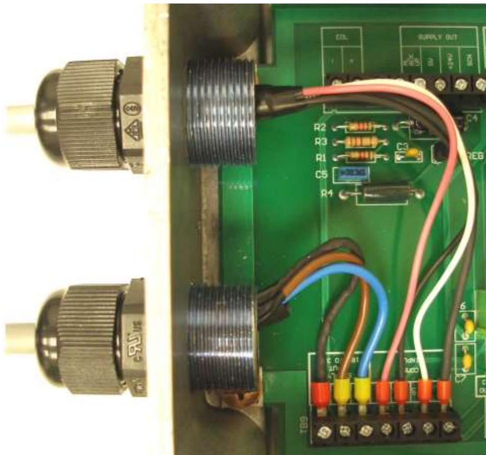
Figure 29 Junction Box Power cable & Communications terminal connections.
