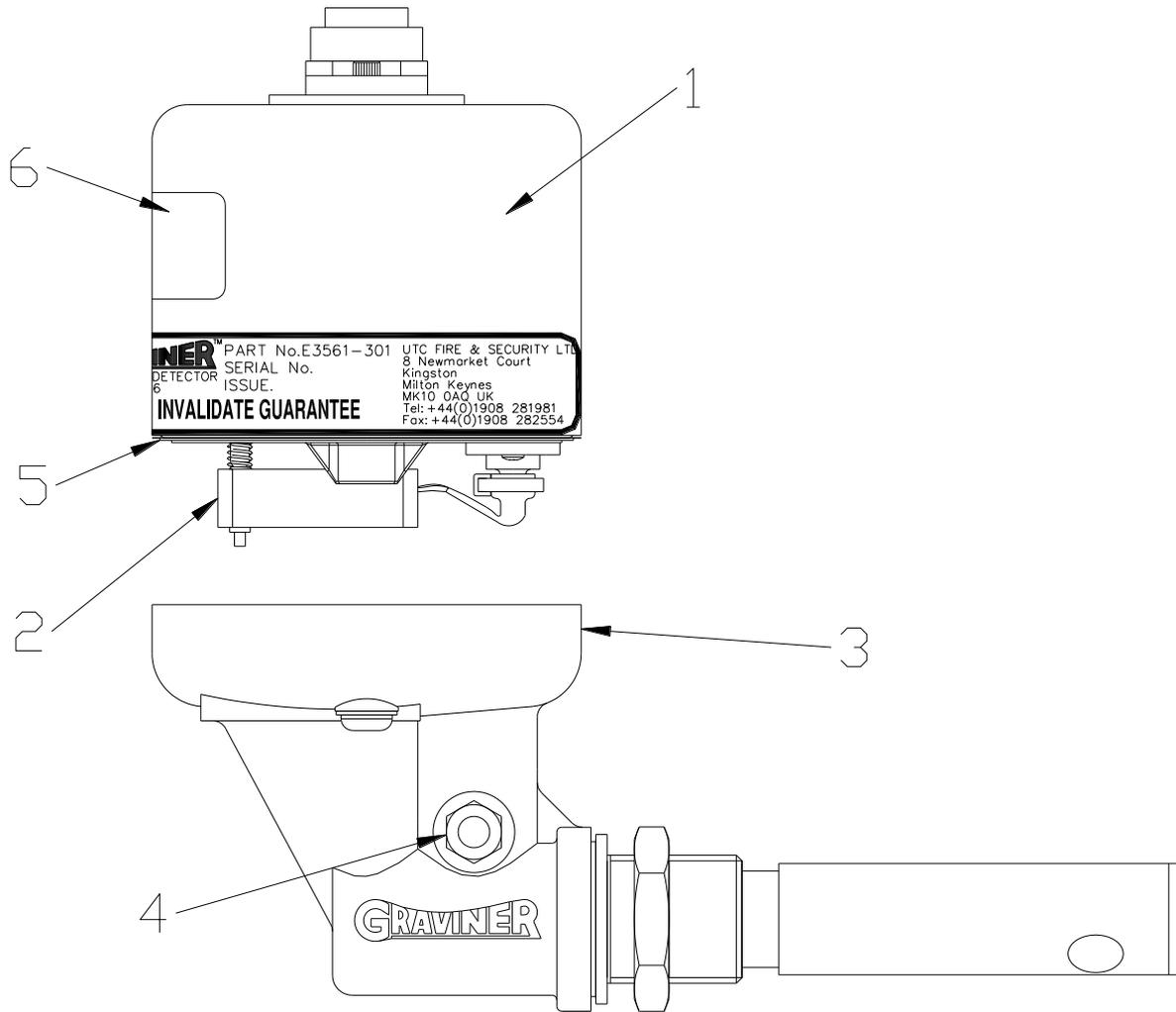
Figure 162 Detector Spares
