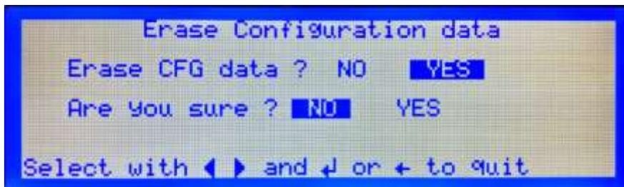
Figure 111 Confirm Configuration Reset.
