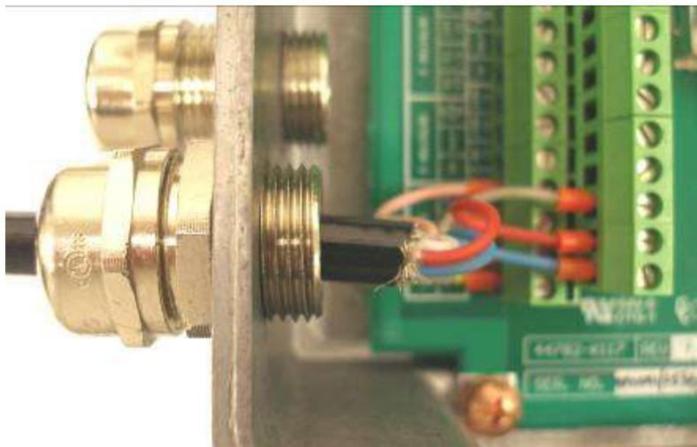
Figure 33 Close-up of Detector cable, EMC Gland assembly
