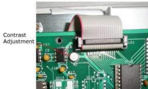
Figure 157 Contrast Adjustment
