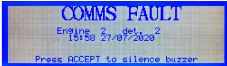
Figure 137 Communications Fault
