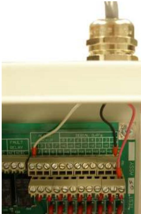
Figure 26 Communications cable connections to Interface Board
