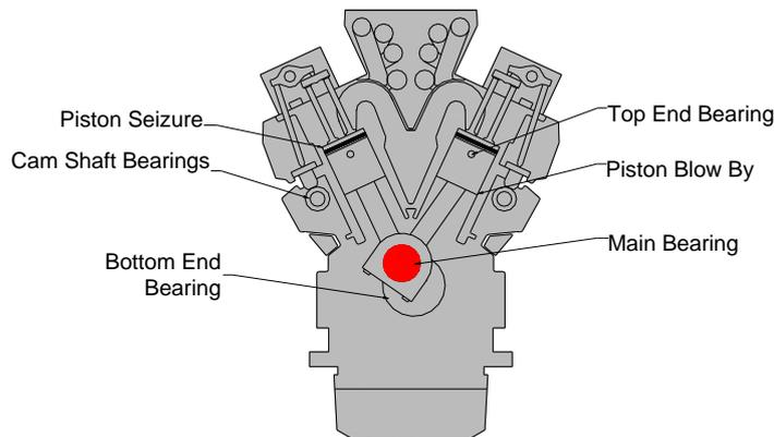
Figure 2 Areas of Failure – 4 Stroke Engine
